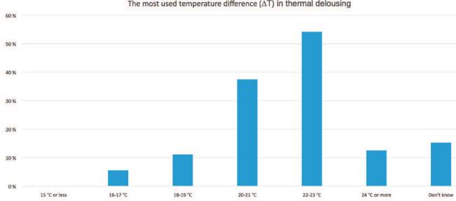
The most used temperature difference ( $\Delta T$ ) in thermal delousing
